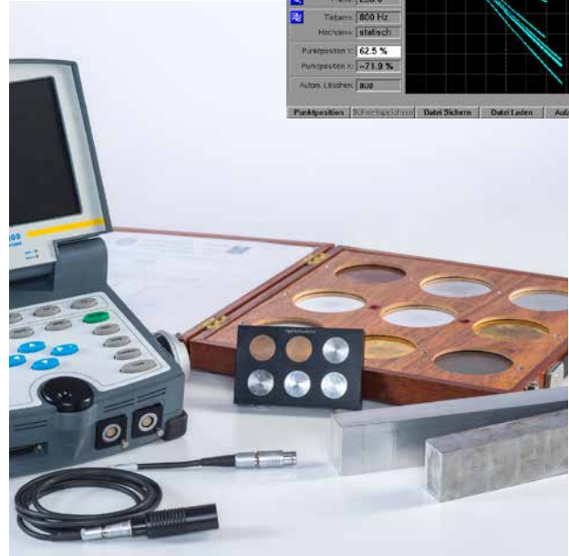
Conductivity test – Measurement of the conductivity of non-ferromagnetic metals and coating thickness measurement
