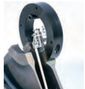
Manipulator-compatible probe, adapted for inspecting complex geometry
