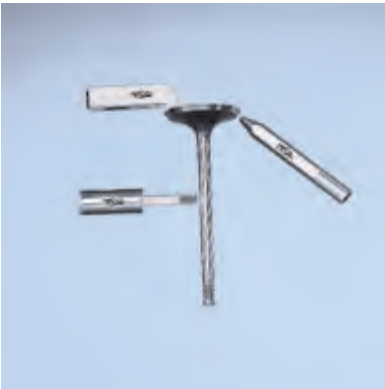
Pinholes, cracks and welding defects on multi-fuel valves
