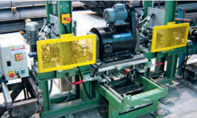
Steel bar inspection with EC100 rotor
