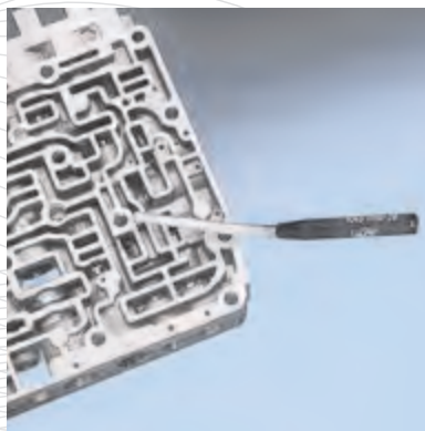
Crack detection on complex structures
