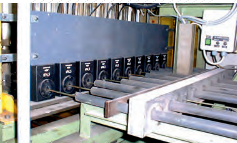
Multi-channel inspection with coils
