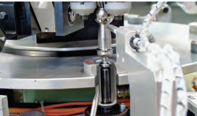
Fully-automatic crack detection on ball studs
