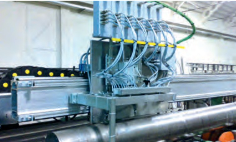
Tube inspection with probe array
